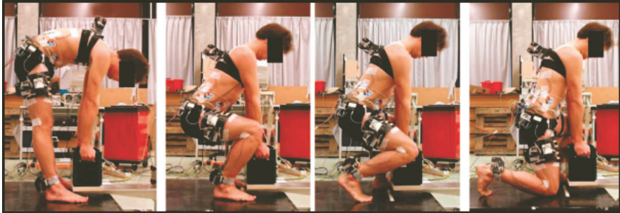
Figure 1: Typical lab study investigating the effect of lifting technique on spinal loading
