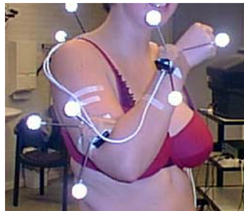
Fig. 2. Attachment of Vicon markers and inertial sensing units to the forearm and upperarm. Sensors are adhered to the segment using double sided adhesive tape and secured using Leukoplast.
